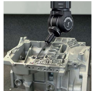
REVO 5-axis measurement system
