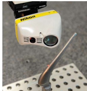
High accuracy LC15Dx laser scanner
