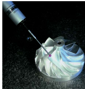
High speed SP25 scanning probe
